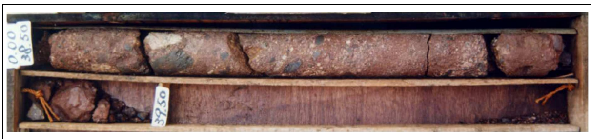
Figure 4.4 Poorly-sorted, Purplish Red, Conglomerate and Sandstone Encountered in an Offshore Drillhole (no. 19102/ODB/4; 807169E, 831378N) in Deep Bay
