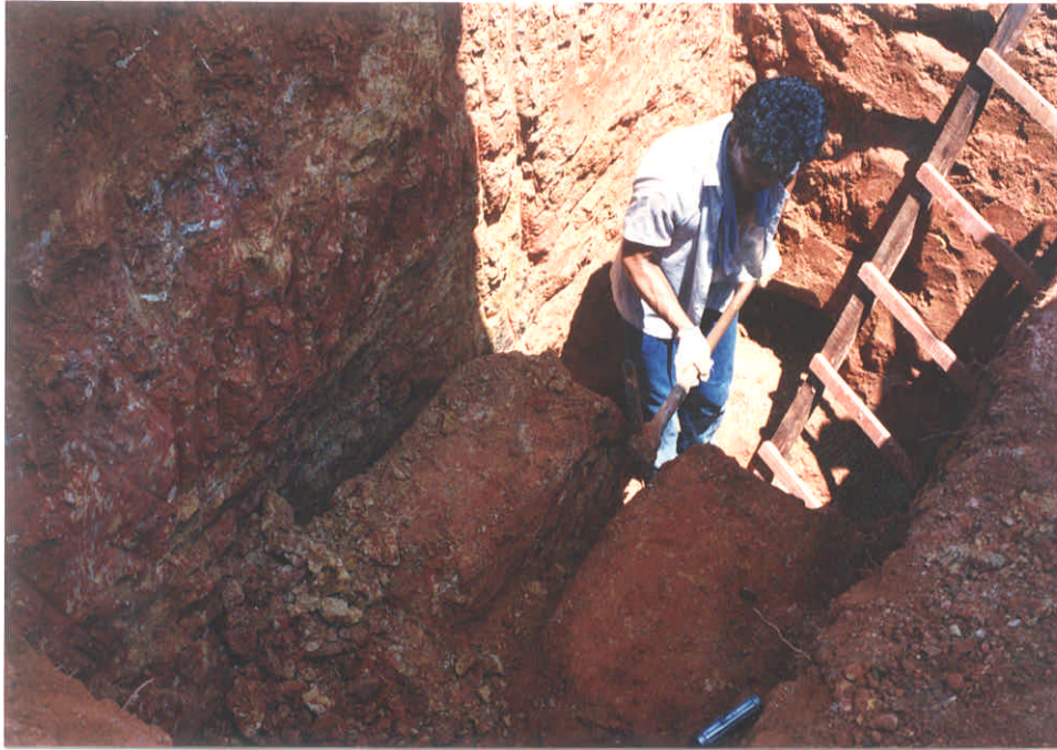
Plate A5 - Sampling Operation - Hand Trimming of Block Sample
