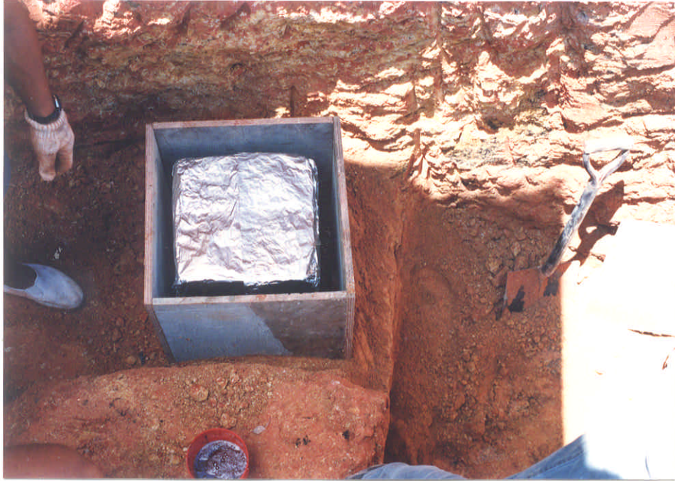
Plate A7 - Sampling Operation - Sample Box in Place
