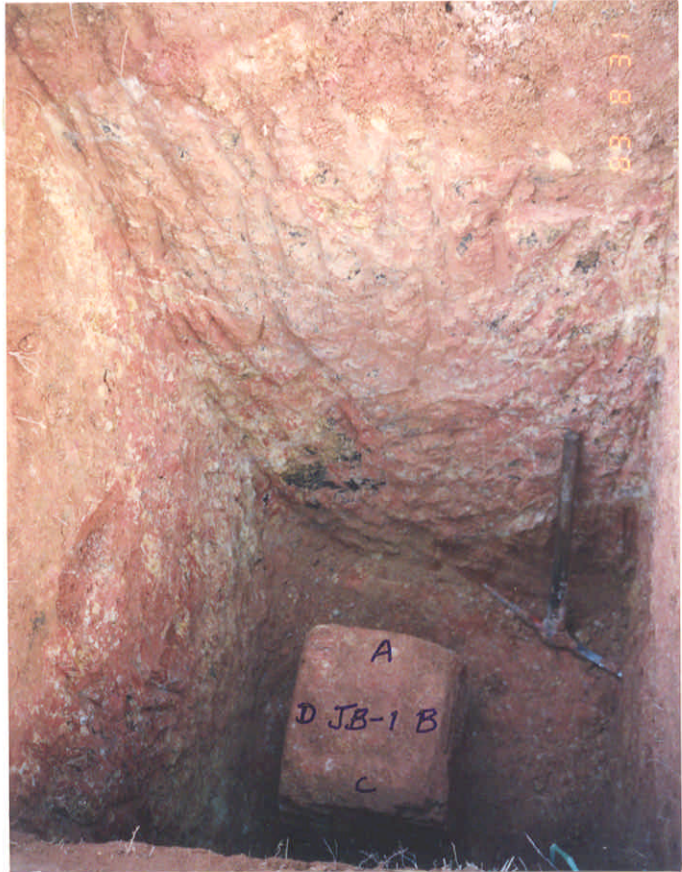
Plate A9 - Sample JB-1 and Faces A & D of the Trial Pit TP1
