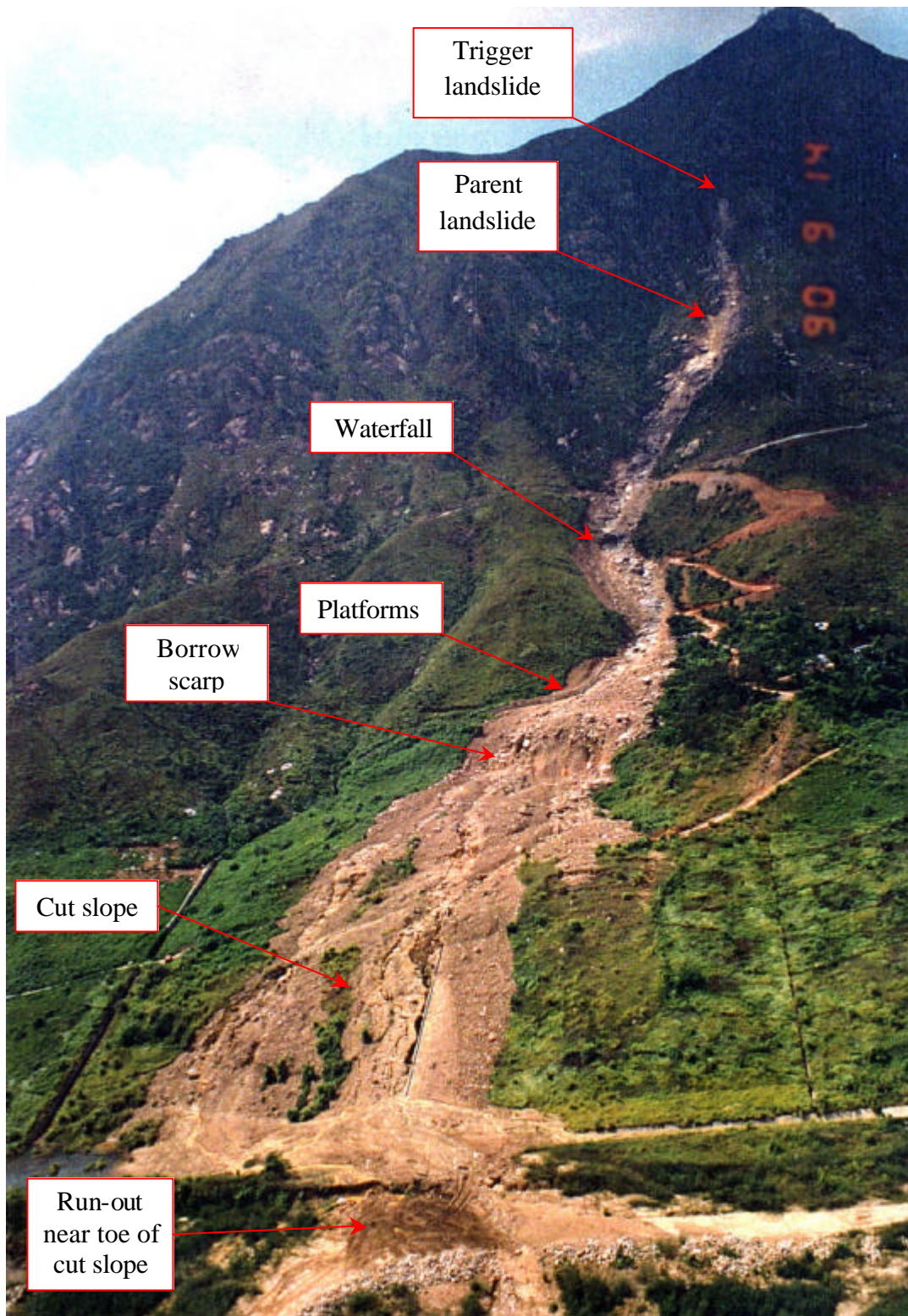
Plate 5 - Oblique Aerial View of the 1990 Tsing Shan Debris Flow (Photograph taken on 14 September 1990)
