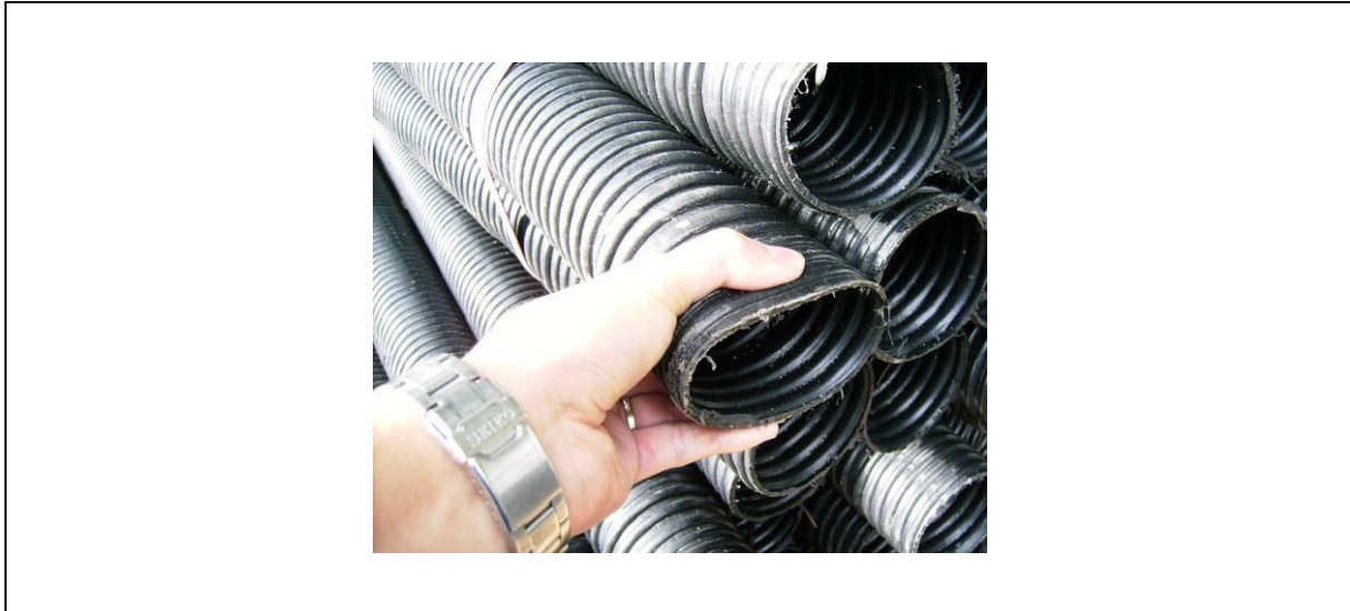
Figure 7.1 Oval Shape of Corrugated Sheathing Resulting from Squeezing by Hand
