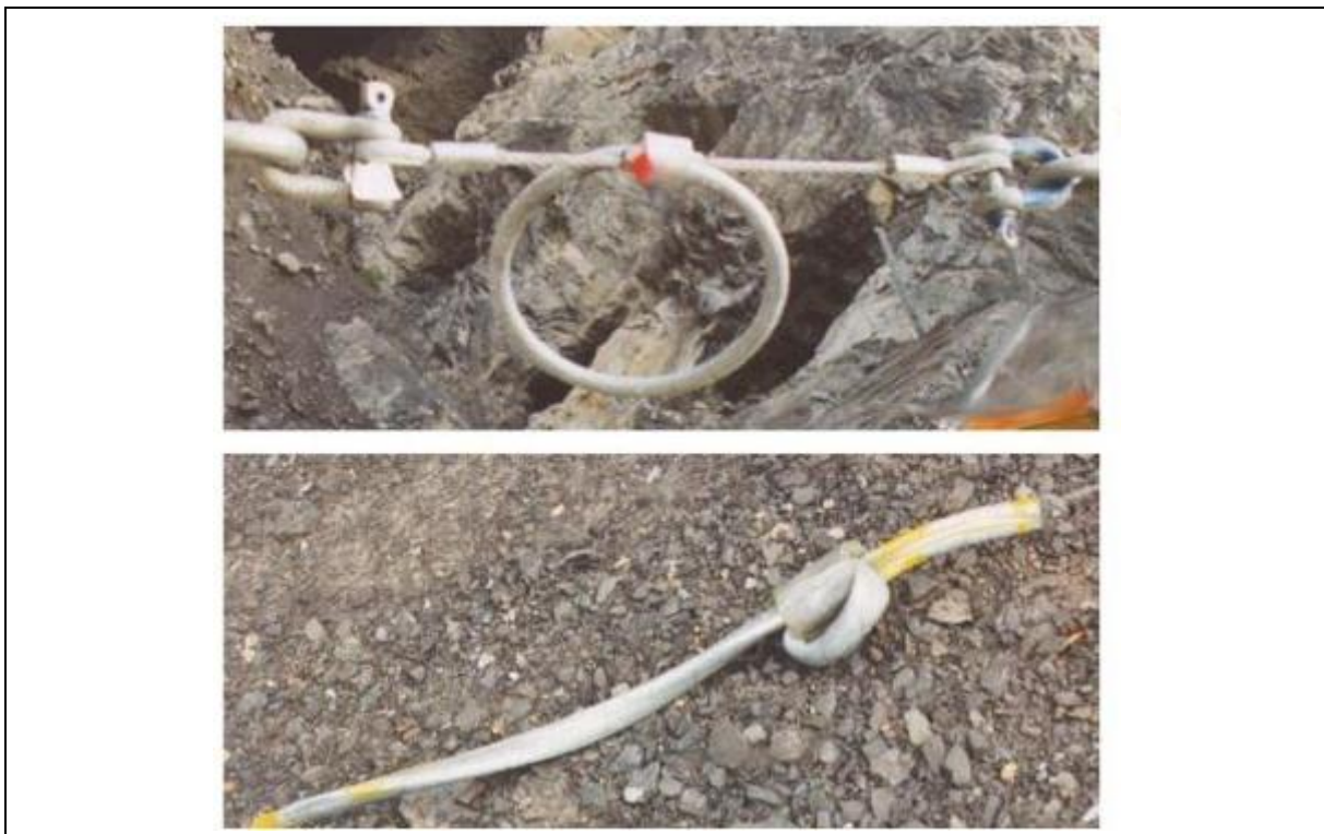
Figure A5 (Top) Brake Ring in its Original Shape; and (Bottom) Deformed Brake Ring Subject to Tension Load
