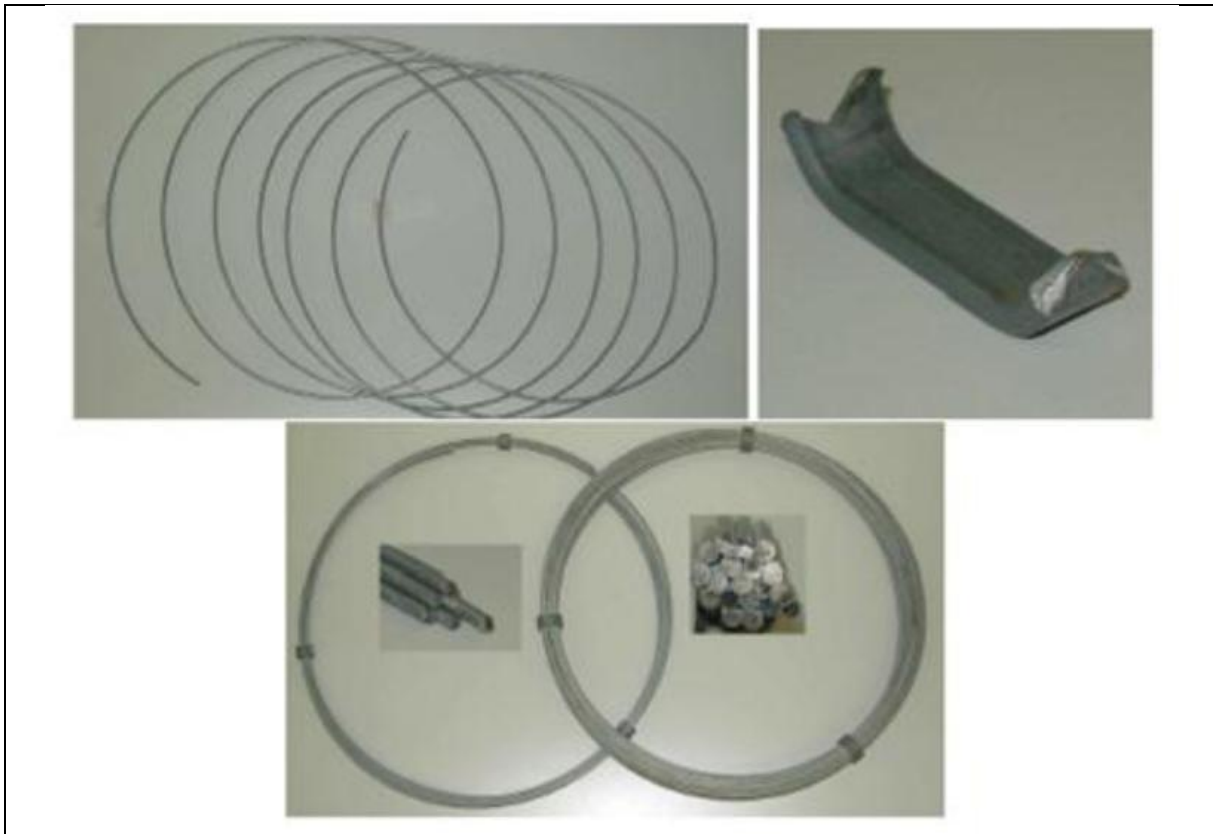
Figure A4 Windings of Steel Wires Forming Rings
