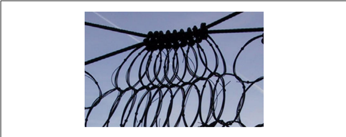
Figure 2.1 Shackles Carrying the Barrier Net Move towards the Middle of Cable after Rockfall Impact (Volkwein, 2004)
